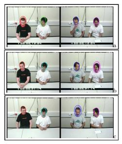
Fig. 3. Multi-object speaker tracker in the meeting room. The speaking status is inferred for each participant, a speaker is shown with a double ellipse.
